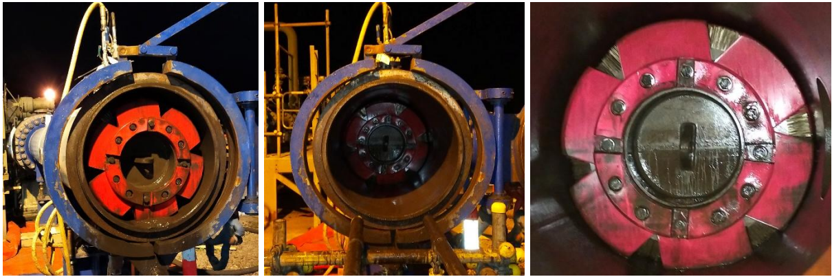
Figure 6: pigs in receiver, very little residue evident
