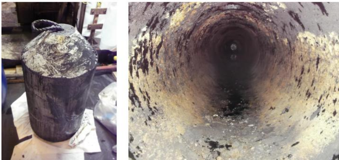
Figure 1: Pig Run No. 1, the foam pig removed minimal debris as intended and left the pipeline free of hydrocarbon gas and nitrogen filled.
